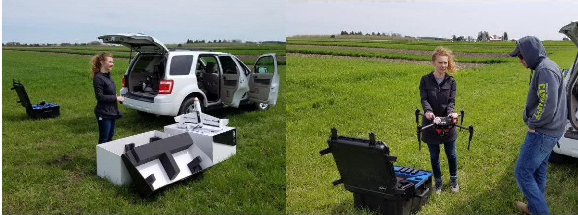
Figure 1. Deployment of rotor-type and hybrid fixed-wing Unmanned Aerial Vehicles for remote sensing data collection in Wisconsin, U.S.A. Undergraduate and graduate students obtained Remote Pilot Licenses from the U.S. Federal Aviation Administration in order to conduct this research.
